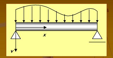
$$\Pi = U - W = \int_0^l \left| \frac{EI}{2} \left( \frac{d^2 v}{dx^2} \right)^2 - q(x)v \right| dx$$
