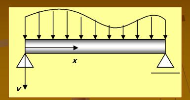
$$\frac{\partial F}{\partial v'} - \frac{d}{dx} \left( \frac{\partial F}{\partial v''} \right) = -\frac{d}{dx} (EIv'') = Q_x$$
