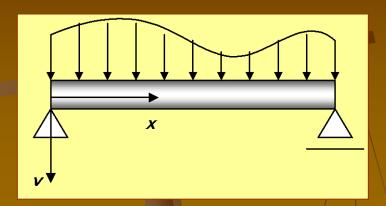
$$\left| \Pi = U - W = \int_0^l \left| \frac{EI}{2} (v'')^2 - q(x)v \right| dx \right|$$
