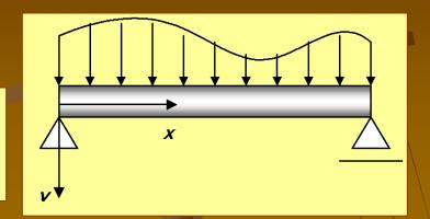
$$U = \int_0^l \left( \int \frac{1}{2} \sigma_x \varepsilon_x b dy \right) dx = \int_0^l \left( \int \frac{1}{2} E \varepsilon_x^2 b dy \right) dx$$
