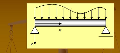
$$\left| \frac{\partial \Pi}{\partial a} = \int_{x} \left\{ EIa \left( \frac{\pi}{L} \right)^{4} \sin \left( \frac{\pi}{L} x \right) - q \right\} \sin \left( \frac{\pi}{L} x \right) dx = 0$$
